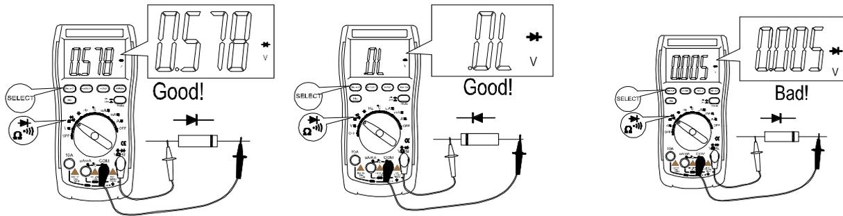
D) Connect the RED test lead to the positive pole of the tested diode, BLACK test lead to the negative pole.
