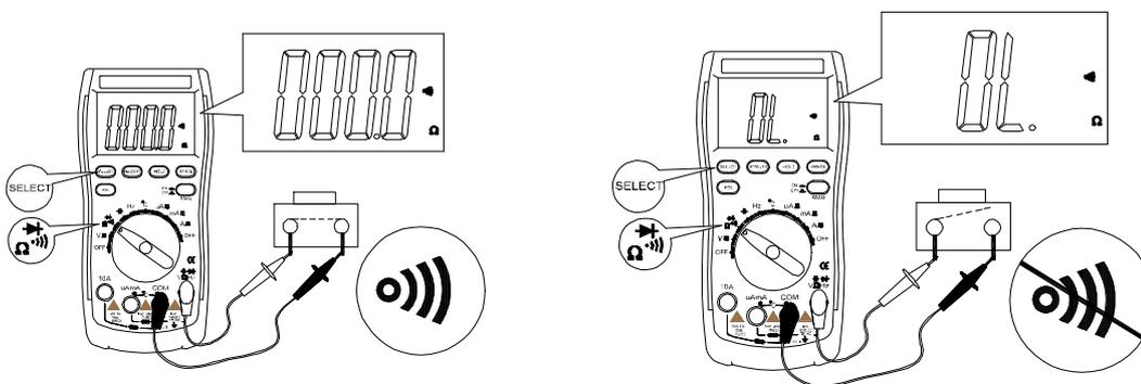
D) Connect the test lead to the two ends of tested circuit in parallel.
