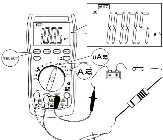
B) Insert the red and black test lead separately to  $\mu A$  mA and COM input terminal.
